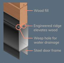
Integrated water drainage protects wood
